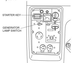
Figure 19. GeneratorLamp Switch
